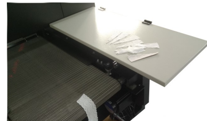
Cut pieces Pickup zone with sorting table
